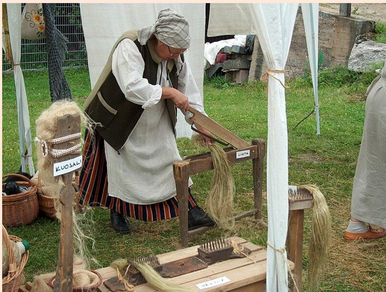
Brake Board in Use -Breaking flax during Anttila Harvest Market in Tuusula, Finland
